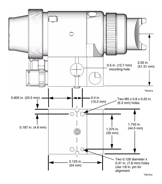
Fig. 29: Manifold Mounting Hole Layout
